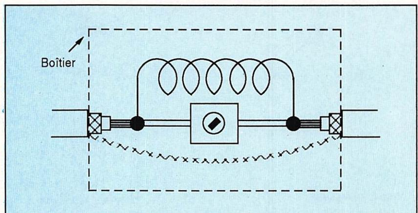
Figure 2 - Filter "Bouchon".
