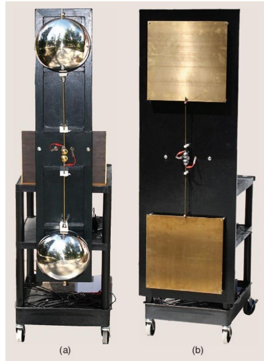
**FIGURE 1.** Two replicas of Hertz's antennas mounted on fiberglass carts: (a) an SLD-1 and (b) a PLD.
